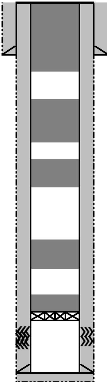
8-21-2020: Top off plug. 20 sx Type II to top off 5 1/2" casing.
