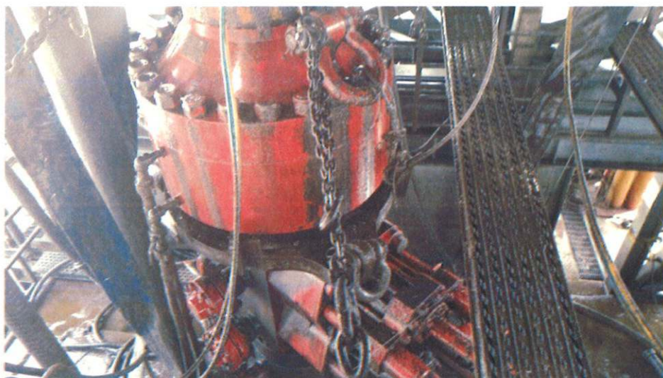
Figure 1: Winch System attached to BOP Stack
