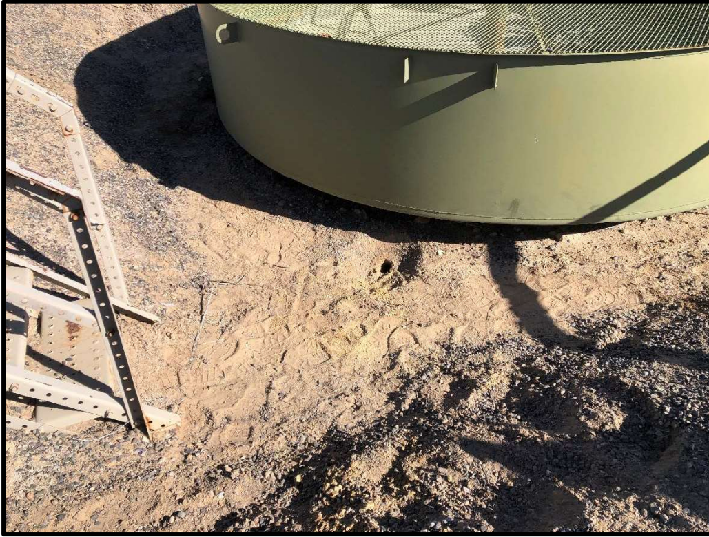
Photo 1: Above - Collection point of S-HA-40", advanced at ~ 25° via hand auger from beneath the above-ground tank.
