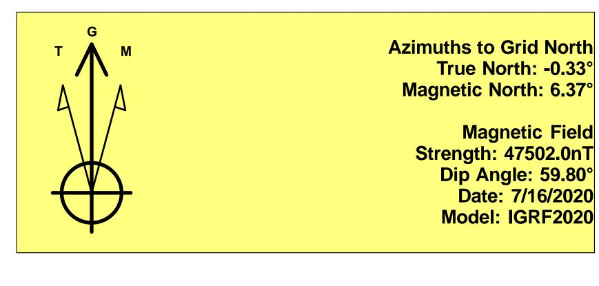
To convert a Magnetic Direction to a Grid Direction, Add 6.37° To convert a Magnetic Direction to a True Direction, Add 6.71° East To convert a True Direction to a Grid Direction, Subtract 0.33°
