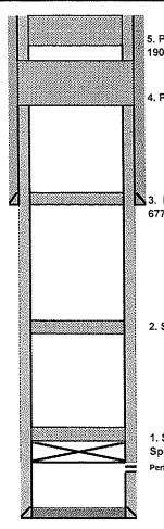
5. Perf'd csg @ 140'. Pressured up on perfs to 500 PSi. Spotted 25 sx class C cmt @ 190' & circulated to surface.
