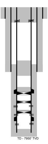
17-1/2" hole @ 535' 13-3/8" csg @ 535' w/ 1400 sx-TOC-Surf-Circ.
