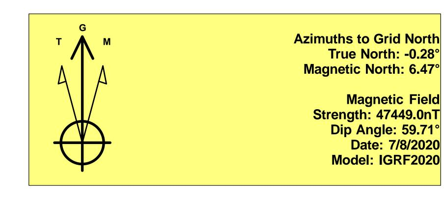
To convert a Magnetic Direction to a Grid Direction, Add 6.47° To convert a Magnetic Direction to a True Direction, Add 6.75° East To convert a True Direction to a Grid Direction, Subtract 0.28°
