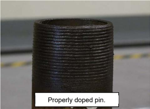
2. If threads are cleaned on racks, new dope shall be applied in a light, even coat to both pin and coupling threads. See Comment No. 1 above for description of sufficient thread compound. Clean thread protectors shall be re-applied to freshly doped pin and coupling threads unless the casing run is imminent (no more than a few hours) to avoid contaminating exposed thread compound.
