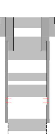
Well Type Oil (ACTIVE) Isolate FW 26 sacks Class C cement Isolate 5-1/2" shoe, Yates Cmt from 1050' to 630' 55 sacks Class C cement **Isolate San Andres** Cmt from 1920' to to 1770' 50 sacks Class C Isolate existing perforations Cmt from 2605' to 2505' minimum Pump excess cement to account for losses to perforations. Theoretical = 33 sacks, pump 200 sacks Original perforations 2605' - 09', 2580' - 86' 50 sack Cement: 3500' - 3370'
