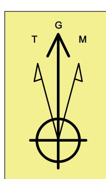
**Azimuths to Grid North** True North: -0.22° Magnetic North: 6.59°
