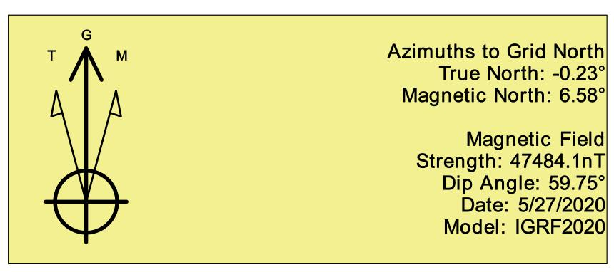
To convert a Magnetic Direction to a Grid Direction, Add 6.58° To convert a Magnetic Direction to a True Direction, Add 6.81° East To convert a True Direction to a Grid Direction, Subtract 0.23°
