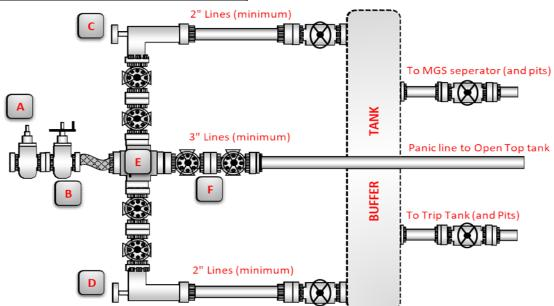
Choke Manifold Installation Checklist: The following items must be verified and checked off prior to pressure testing BOP equipment
