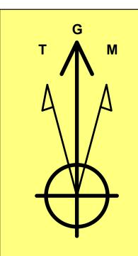
**Azimuths to Grid North** True North: -0.35° Magnetic North: 6.41°
