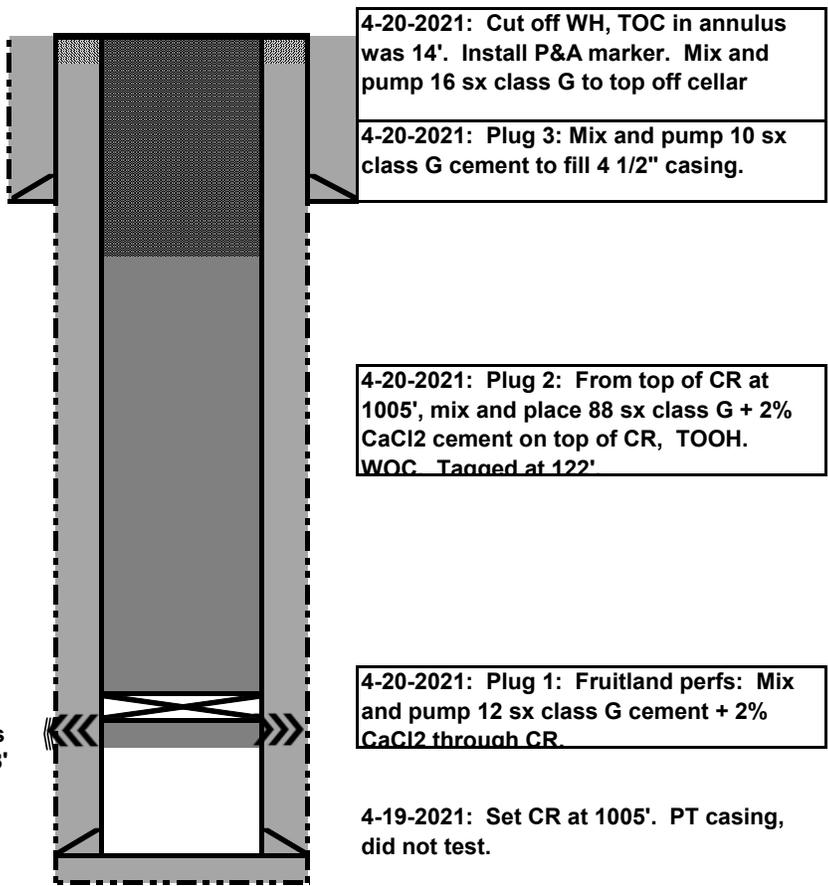
4-20-2021: Cut off WH, TOC in annulus was 14'. Install P&A marker. Mix and pump 16 sx class G to top off cellar
