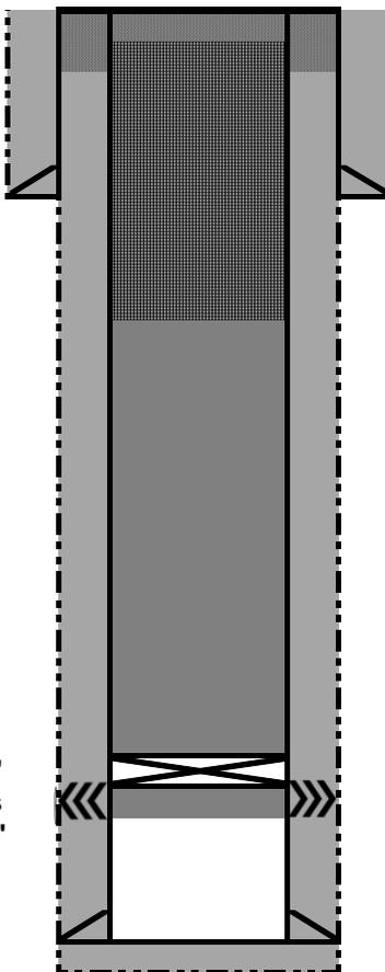
12-23-2020: Tag TOC in casing at 2'. TOC in annulus at 30'. Install P&A marker, top off with 25 sx Class G cement.
