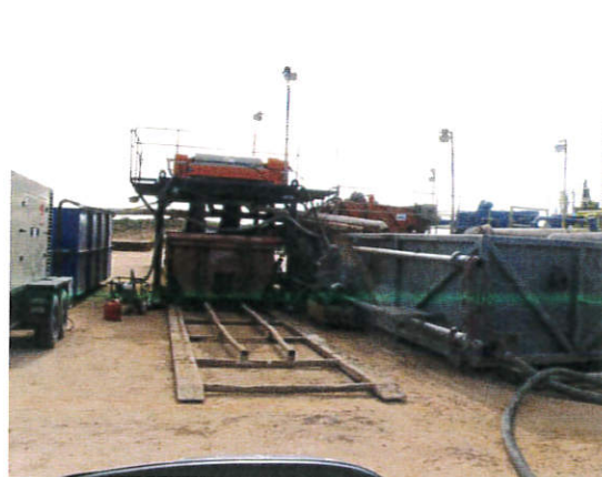
Above: Centrifugal Closed Loop System
