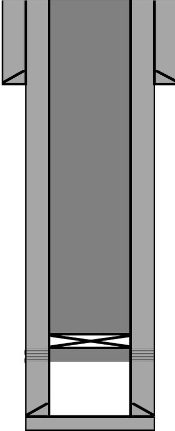
4-28-2021: TOC at WH. Topped off with 21 sx. Cut off WH. TOC in annulus was at 20'. Installed P&A marker. Mixed and pumped 25 sx cement to top off cellar.
