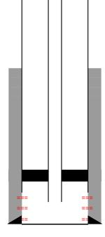
Completion Equipment in hole: Halliburton R-4 inj packer set at 2477' 2-3/8" plastic coated tubing
