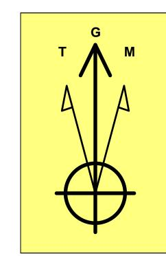
**Azimuths to Grid North** True North: -0.36° Magnetic North: 6.23°
