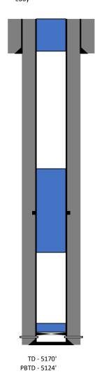
EOT @ 554'. PUMPED 45SX CL C CMT TO SURFACE. VERIFIED.
