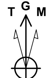
Azimuths to Grid North True North: -0.09° Magnetic North: 6.85° Magnetic Field
