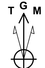
Azimuths to Grid North True North: -0.09° Magnetic North: 6.85°
