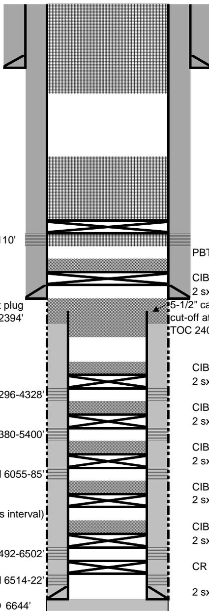
**Plug 2: Nacimiento, surface casing shoe, surface: Mix and pump sufficient cement to bring cement from 481' to surface.**
