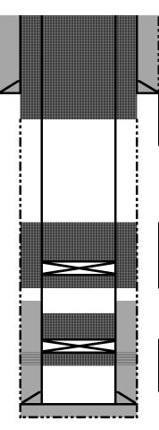
Plug 3: Nacimiento, surface casing shoe, surface: Perf holes at 291'. Tie onto 5-1/2" casing. Mix and pump sufficient cement to bring cement to surface inside and outside 5-1/2" casing.
