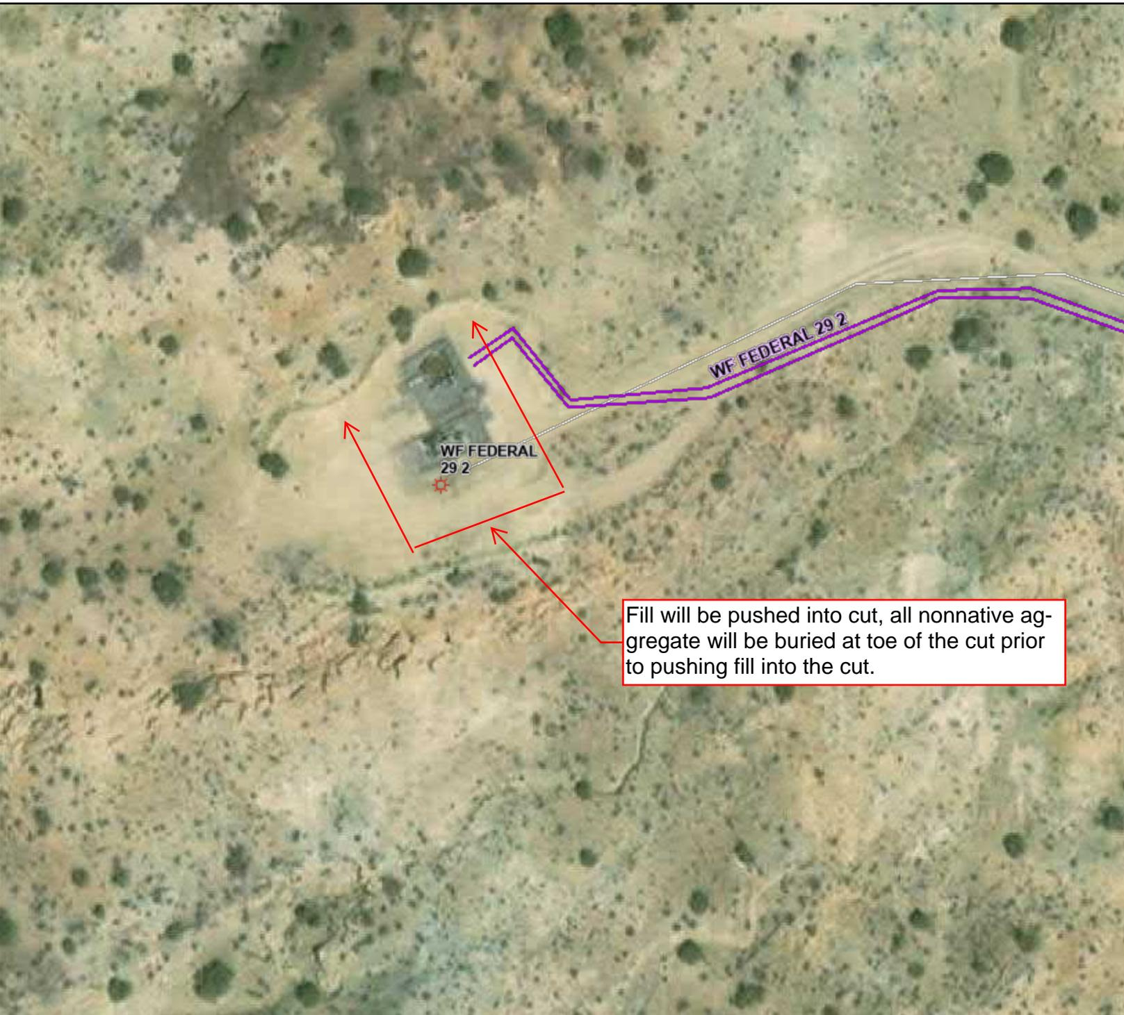
Fill will be pushed into cut, all nonnative aggregate will be buried at toe of the cut prior to pushing fill into the cut.
