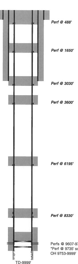
17-1/2" hole @ 438' 13-3/8" csg @ 438' w/ 370sx-TOC-Surf-Csg
