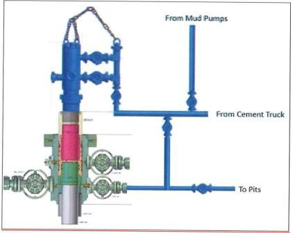
Wellhead diagram during offline cementing operations
