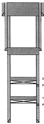
13 3/8 48# CSG @ 200 4. Perf'd @ 223'. Pressured up on perfs to 500 PSI. ND BOP. Spotted 40 sx class C cmt @ 273' & circulated to surface.
