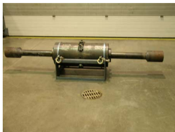
TEST SPECIMENS INSIDE THE EXTERNAL PRESSURE CHAMBER
