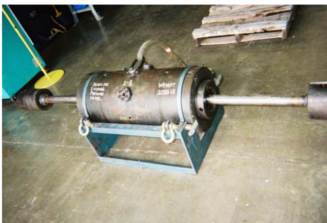
TEST SPECIMENS INSIDE THE EXTERNAL PRESSURE CHAMBER
