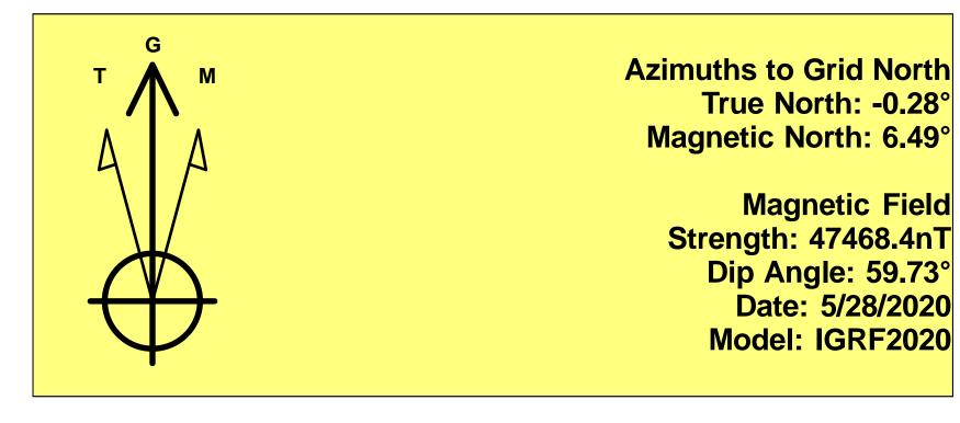
To convert a Magnetic Direction to a Grid Direction, Add 6.49° To convert a Magnetic Direction to a True Direction, Add 6.77° East To convert a True Direction to a Grid Direction, Subtract 0.28°
