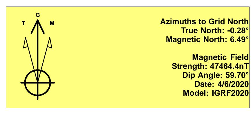
To convert a Magnetic Direction to a Grid Direction, Add 6.49° To convert a Magnetic Direction to a True Direction, Add 6.77° East To convert a True Direction to a Grid Direction, Subtract 0.28°
