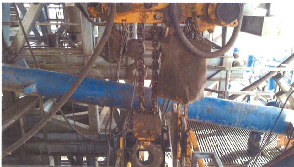
Figure 2: BOP Winch System
