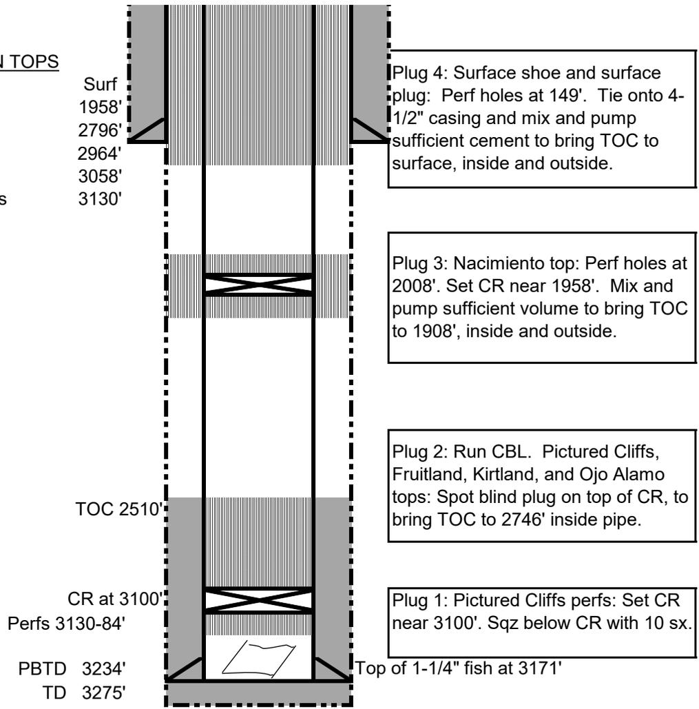
Plug 4: Surface shoe and surface plug: Perf holes at 149'. Tie onto 4-1/2" casing and mix and pump sufficient cement to bring TOC to surface, inside and outside.
