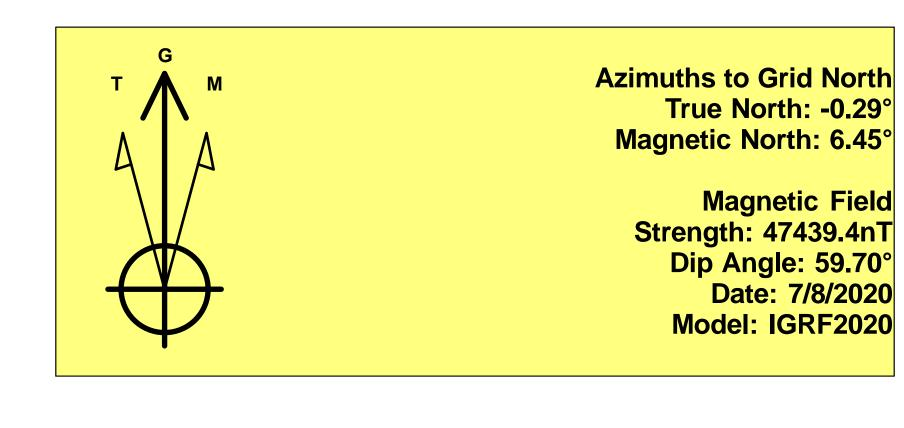
To convert a Magnetic Direction to a Grid Direction, Add 6.45° To convert a Magnetic Direction to a True Direction, Add 6.74° East To convert a True Direction to a Grid Direction, Subtract 0.29°
