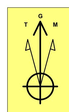
Azimuths to Grid North True North: -0.28° Magnetic North: 6.46°
