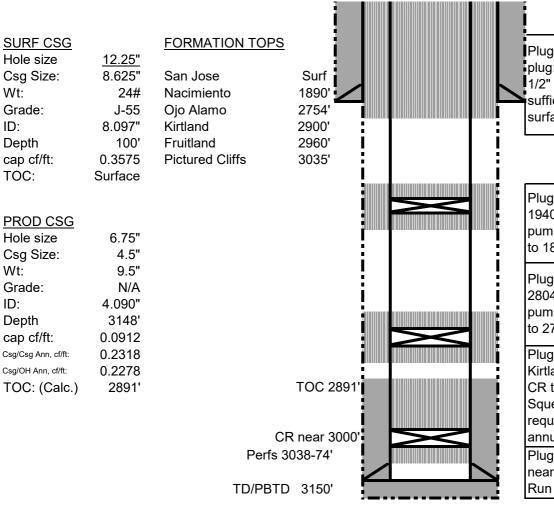
Plug 5: Surface shoe and surface plug: Perf holes at 150'. Tie onto 4-1/2" casing and mix and pump sufficient volume to bring cement to surface, inside and outside.
