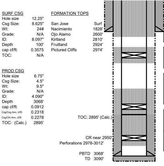
Plug 5: Surface shoe and surface plug: Perf holes at 150'. Tie onto 4-1/2" casing and mix and pump sufficient cement to bring TOC to surface, inside and outside.
