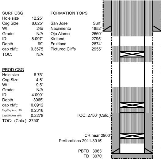
Plug 5: Surface shoe and surface plug: Perf holes at 149'. Tie onto 4-1/2" casing and mix and pump sufficient cement to bring TOC to surface, inside and outside.
