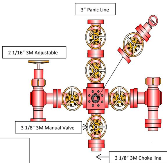
**Choke Diagram for a 3,000psi system**
