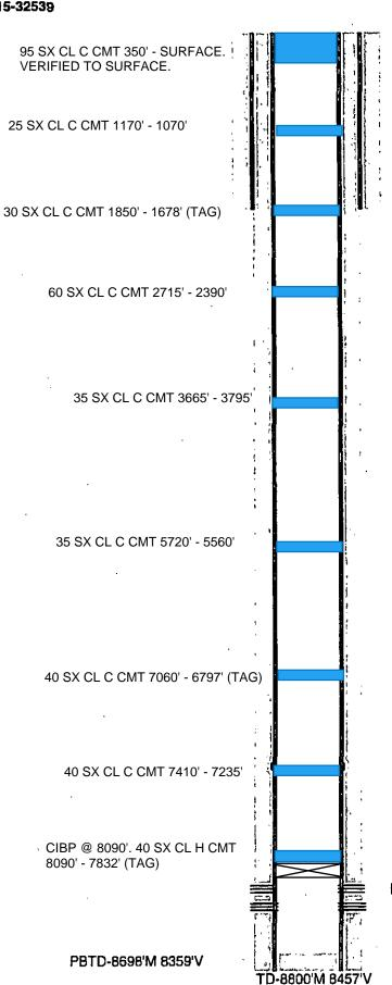
12-1/4" hole @ 1800' 9-5/8" csg @ 1800' w/ 1300sx-TOC-Surf-Circ
