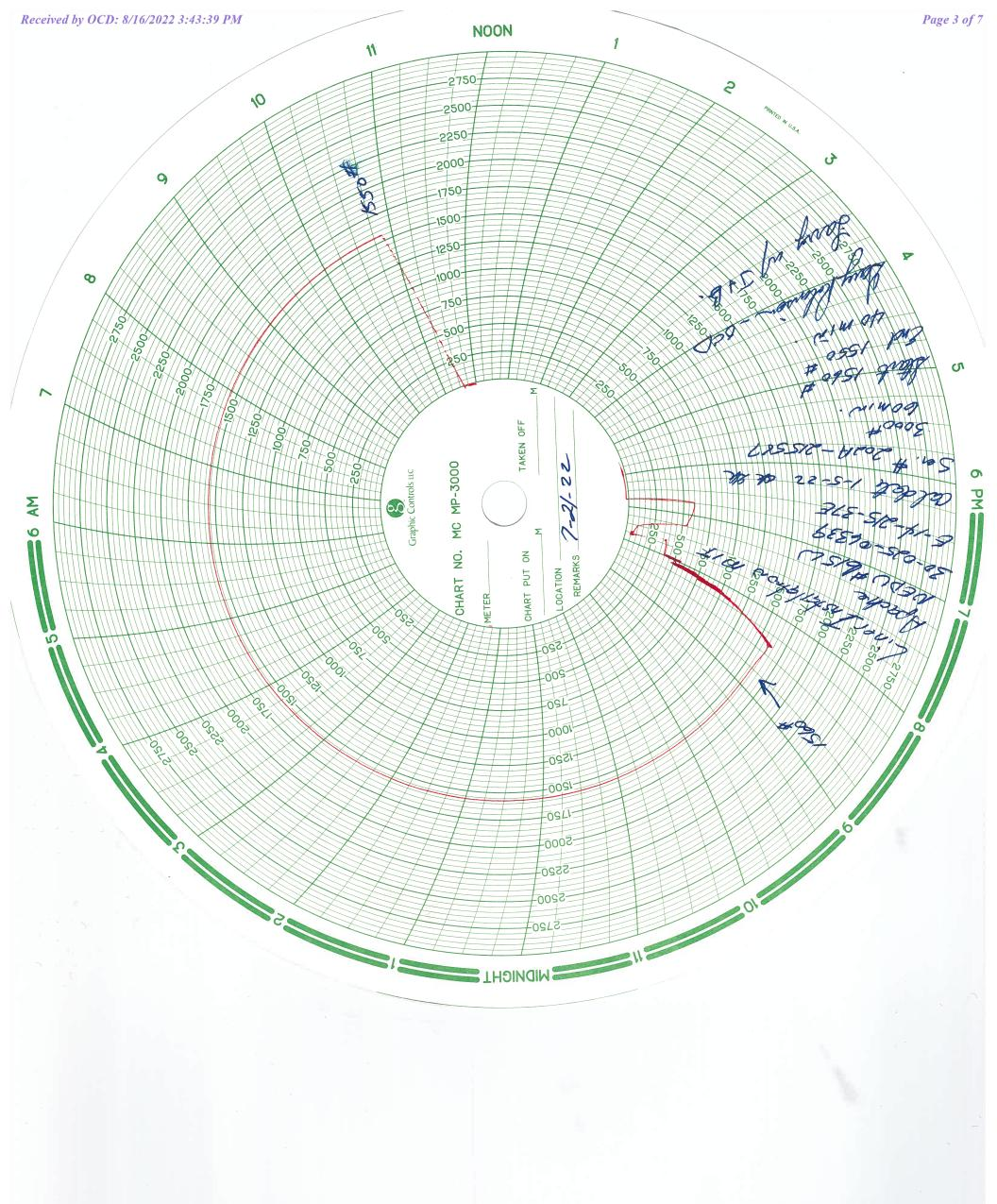
Please find the compiled information from the step rate test on the NEDU 615W. This job was pumped by Big E Services with Precision Wireline recording downhole data. The break over point occurred at the 1.5 BPM rate with the surface parting pressure at the end of this step being 2,722 psi. This is greater than the current max injection pressure at surface of 1,375 psi authorized for the Northeast Drinkard Unit.
