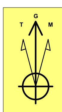
**Azimuths to Grid North** True North: -0.33° Magnetic North: 6.39°
