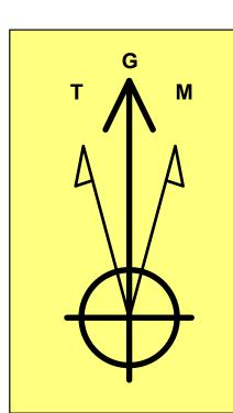
**Azimuths to Grid North** True North: -0.33° Magnetic North: 6.39°
