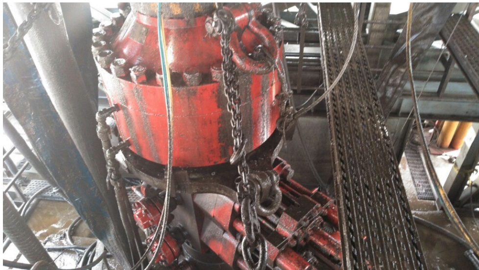
Figure 1: Winch System attached to BOP Stack
