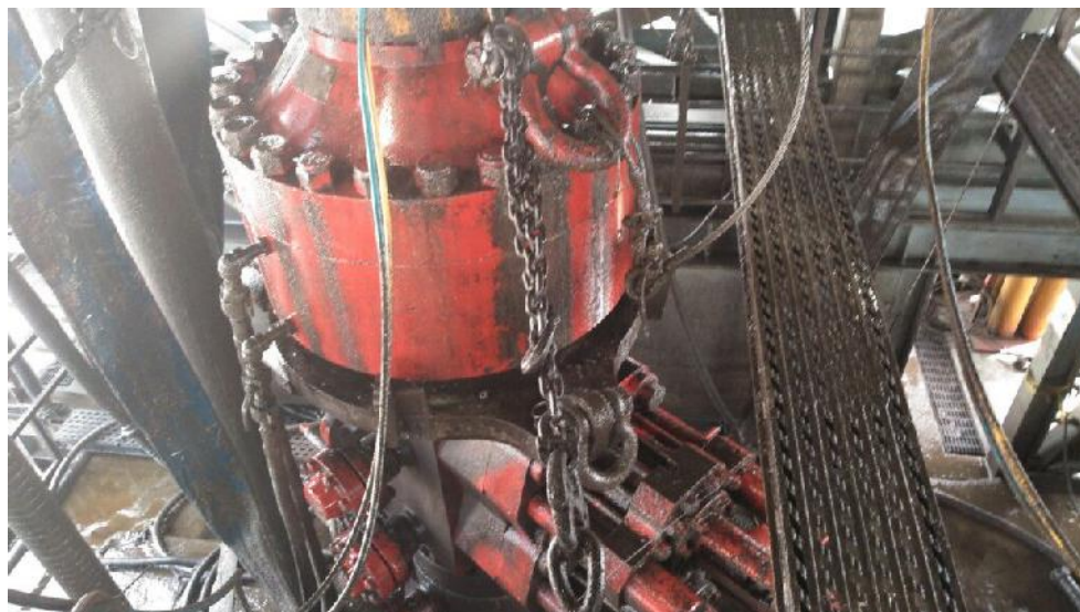
Figure 1: Winch System attached to BOP Stack
