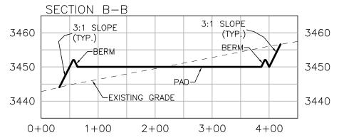
REDWOOD OPERATING LLC GRADING PLAN AND CROSS SECTIONS FOR MALCO B 6 FEDERAL COM 4H SECTION 5, TOWNSHIP 18 SOUTH, RANGE 27 EAST, N.M.P.M. EDDY COUNTY, STATE OF NEW MEXICO
