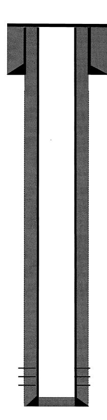
8-5/8" 24# J-55 casing @ 129'. Cemented with 50 sks Type 5 cement w/2% CaCl2 . Circulated 4 bbls cement to surface. Hole size 12  $\frac{1}{4}$ ".
