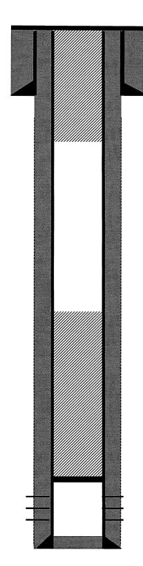
8-5/8" 24# J-55 casing @ 129'. Cemented with 50 sks Type 5 cement w/2% CaCl2 . Circulated 4 bbls cement to surface. Hole size 12  $\frac{1}{2}$ ".
