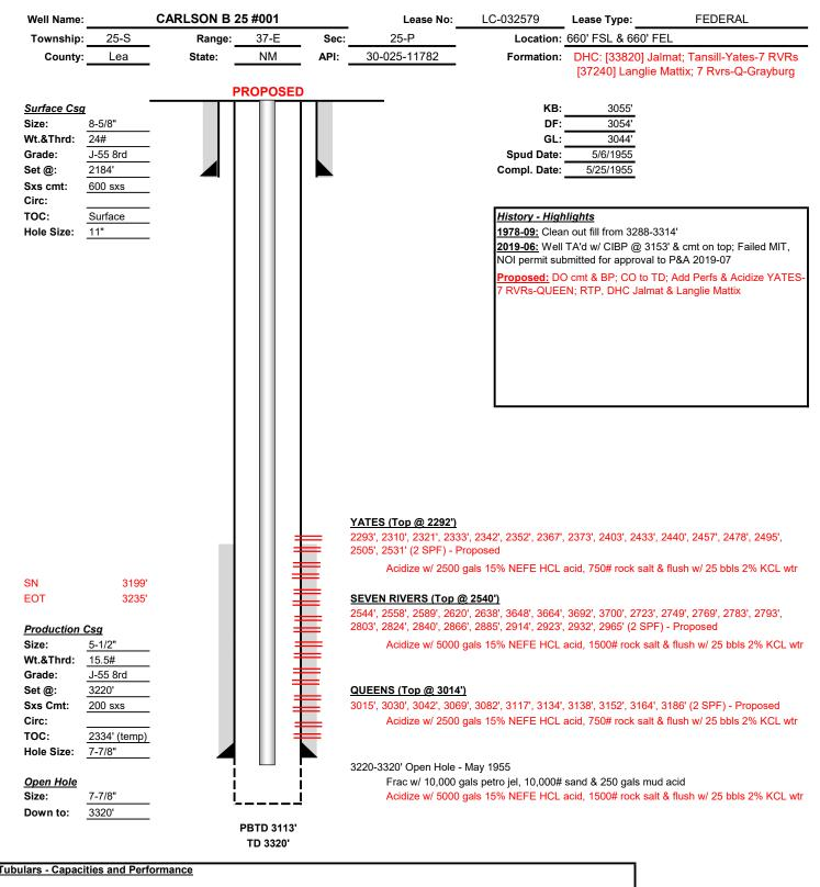
2-3/8" 4.7# J-55 EUE 8rd Tubing (99 jts 2-3/8" tbg, SN, 4' perf sub, MA w/ bull plug)
