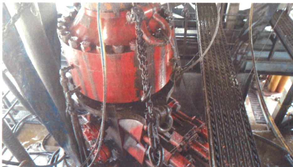
Figure 1: Winch System attached to BOP Stack
