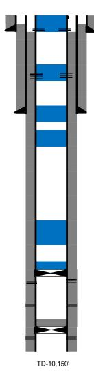
17-1/2" hole @ 450' 13-3/8" csg @ 448' w/ 400sx-TOC-Surf-Circ
